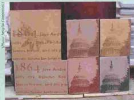
Concrete imprinted using photographic system.
